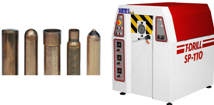
SP-55/SP-110 Tube End Spinning machine for closing, reducing and expanding of copper tubes. - Max tube diameter 108 mm - Max wall thickness 3 mm
